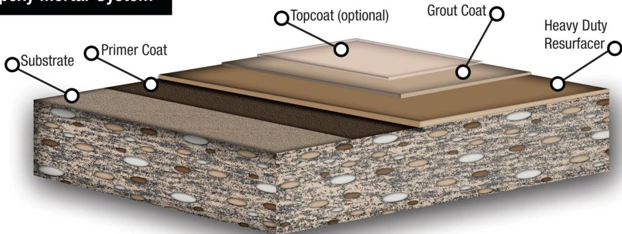
RS-21CF is a Heavy-Duty Epoxy Mortar Flooring System is a troweled, high strength concrete resurfacing material. It is used for low temperature environments (40F-60F) requiring an industrial grade floor or when a concrete floor has sustained damage requiring a 3/16" to 1/4" surface restoration.
