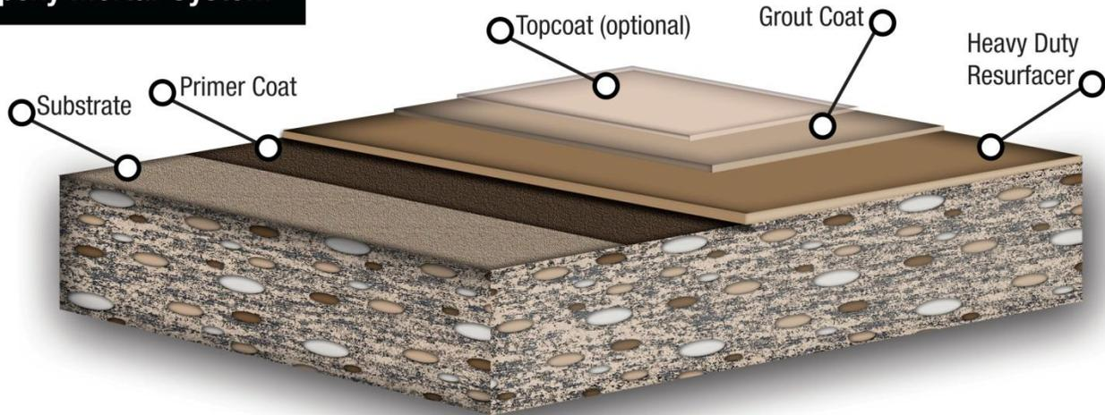
RS-41CR is a Heavy-Duty Acid/Chemical Resistant Epoxy Mortar Flooring System is a troweled, high strength concrete resurfacing material. It is used for environments requiring an industrial grade protective floor or when a concrete floor has sustained damage requiring a 3/16” to 1/4” surface restoration.
